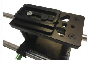
2. Slide the silver rods through the mounting holes on the camera riser. Use the green tabs to open the mounting holes if sliding the rods through is difficult. Tighten the tabs once your rods are inserted.
