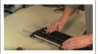
Attach your tripod heads wedge plate onto the bottom of the glide plate. Positioning this plate is critical to balance. The further forward you attach the wedge plate, the more back heavy the system will be once all components are set.
