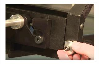
Note: If your beamsplitter frame did not ship with the beamsplitter already installed, remove the top rail of the frame by unscrewing the small screws of either side of the rail. Slide the beamsplitter into place and re-attach the top rail. Your beamsplitter should have a colored sticker on one side. That is the side that faces outward over the monitor.
