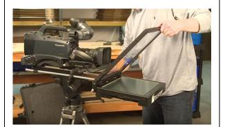
Tilt up the beamsplitter frame and lock into place by turning the two round silver locking knobs. If your frame will not tilt up, turn the knobs so the flat part of the knob is facing up so not to obstruct the frame from fully tilting. Then turn the flat part of the knob down to lock the frame into position.
