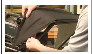
Attach the trifold hood onto the beamsplitter frame using the Velcro strips that are on the edges of the frame and the hood.
