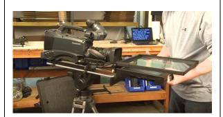
Attach the glide plate to your camera head and put your camera on its plate. Be sure your head is fully locked as the system will be out of balance at this point.
