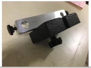
If your counterweight did not come assembled, put the long bolt through the top of the hanger, screw the spinner on the end of the bolt, slide the weight around the bolt and tighten the spinner.
