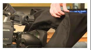
On the back side, using the Velcro, attach the shroud to the hood. Insert the camera lens through the shroud opening and tighten the cord to close up the opening.
