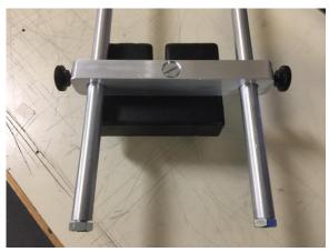
Now, remove the two small retaining bolts at the end of the glide plate rods, slip the weight on, and reinsert the retaining bolts into the glide plate rods.
