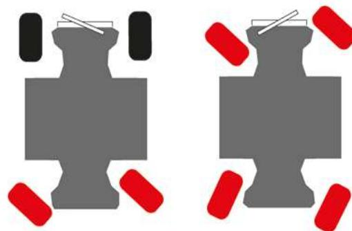
**SWITCH FROM 2- TO 4-WHEEL STEERING BY
